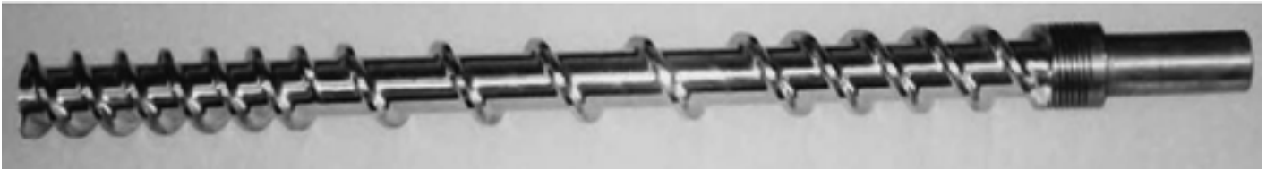
Fig. 1: Screw design of a flight progressive screw for silicone rubber extrusion
