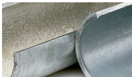
Whenever water is used as a heat transfer or processing medium, salts can deposit to form scale. Dow chelating agents are used successfully to remove calcium and other types of scale and also to prevent scale formation.
