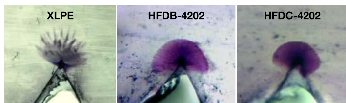
Figure 3: Water tree shape of ENDURANCE™ 4202 TR-XLPEs compared to XLPE at 80X magnification*
