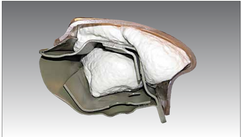
The complex channels in a body cavity are completely sealed by BETAFOAM Renue injected as a liquid to react and fill the intricate space.
