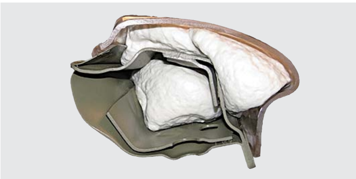
The complex channels in a body cavity are completely sealed by BETAFOAM™ Renue injected as a liquid to react and fill the intricate space.
