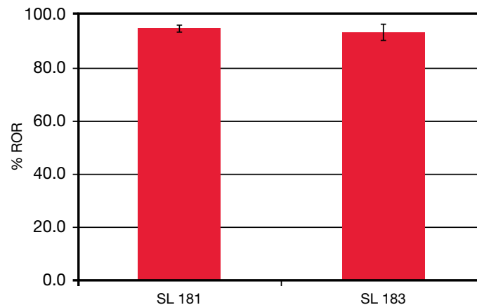
Figure 3. Comparison of rub-off resistance (ROR) of SYL-OFF™ SL 181 Coating and SYL-OFF™ SL 183 Coating, cured at approx. 145°C exit web temperature and 3 sec dwell time.
