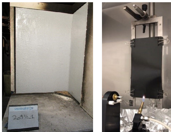
Figure 8: Left: illustration of the EN ISO 13823 test, right: illustration of the EN ISO 11925 small flame test
