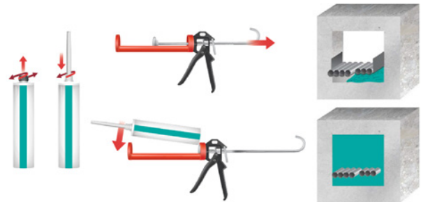
Figure 24: Illustration of the foam installation in a penetration seal in a wall using hand mixed cartridges
