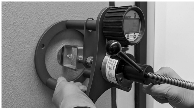
Figure 12. Adhesion test using ASTM D4541
