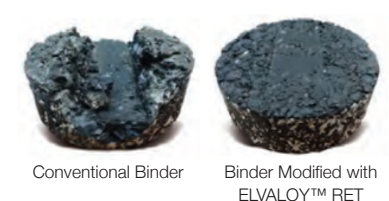
Figure 5: Hamburg Rutting Test Visual Results Conventional Binder vs. Binder Modified with ELVALOY™ RET
