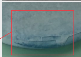
PET bottle flakes sinking in the liquid
