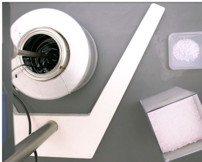
Figure 1: Lab mixer and heating mantle
