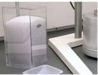
ELVALOY™ RET is supplied to asphalt binder producers in the form of free-flowing pellets for measured conveyance and controlled melt-blending into asphalt in a heated mixing tank.
